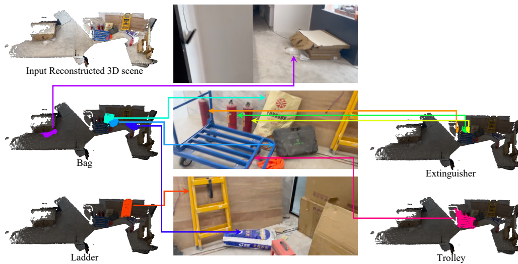
Figure 7: Input text prompt: “bag . ladder . extinguisher . trolley .”. Despite the white plastic bag (with the purple mask) blending into the floor and forming strong geometric continuity, our 2D Instance-Boundary-aware Superpoint (IBSp) enables OVSeg3R to successfully segment it out. Moreover, although the ‘trolley’ class is not present in existing datasets, OVSeg3R is still capable of recognizing and segmenting it. Best viewed in the electronic version or by referring to the 3D segmentation results provided in the supplementary material.
