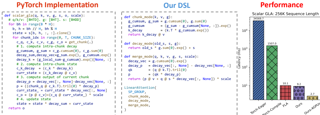
Figure 1: Comparison between PyTorch and our proposed DSL in writing scalar gated linear attention (data type conversion is omitted for simplicity). And the performance comparison of different approaches. Test shape: 32 heads with 128 head dimension. Torch-Eager fails to parallelize the computation, while Torch-Compile also performs poorly. FLA provides expert optimized triton kernels, while program generated by FlexLA offers comparable performance to handwritten kernels with the scalability to distributed environments.
