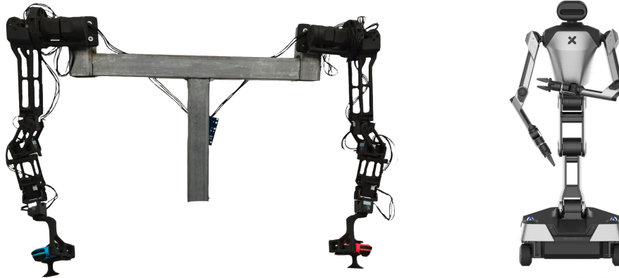
Figure 6: Low-cost JoyLo system and Galaxea R1 robot.
