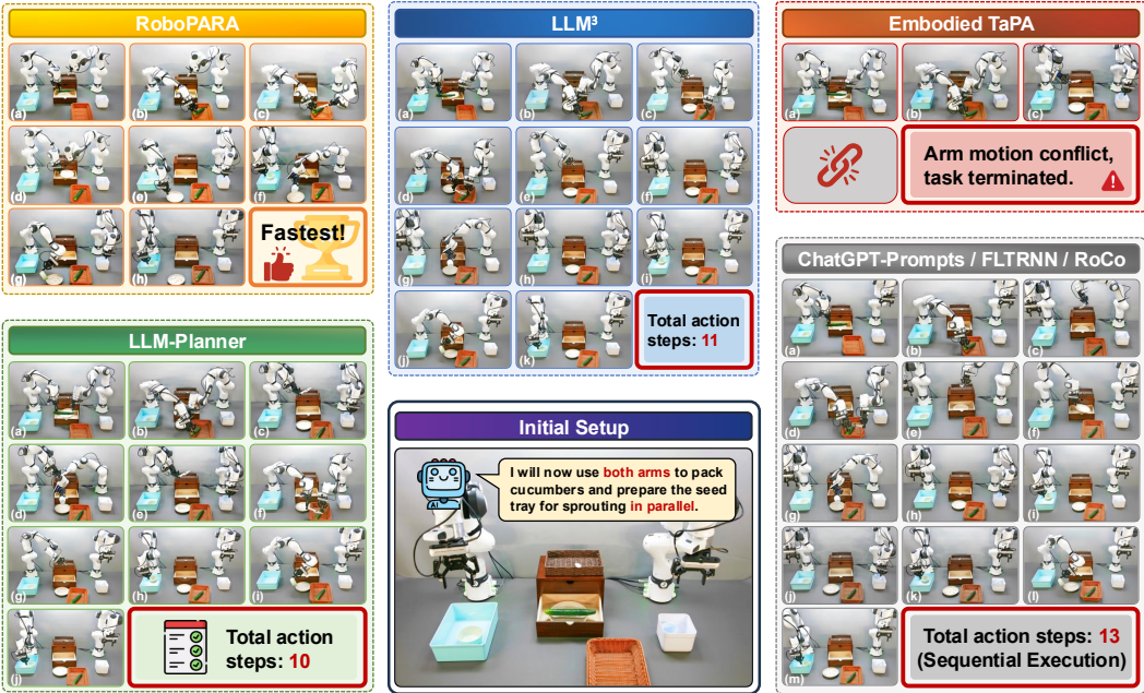
Figure 4: Real-world deployment comparison of RoboPARA and baselines on Franka Research 3 robot in an agricultural greenhouse scene. Voyager is excluded because it cannot provide explicit plans for each arm. See Appendix Sec. E.7.2 for details and specific plans regarding this field test.
