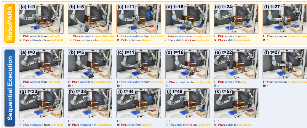
Figure 15: Real-world experiments in factory scene using the UR5e robotic arms. The task is “assemble tool components and prepare electrical tools”. Compared with sequential execution, RoboPARA highlights cross-package parallelism , demonstrating higher-level task planning and integration capabilities.
