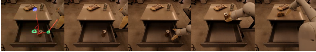
Figure 6: Example trajectory from image generation models. From left to right, the first image shows the overlaid trajectory sketch, and the next 4 images show the rollout conditioned on it. The language instruction is: pick orange can from top drawer and place on counter.
