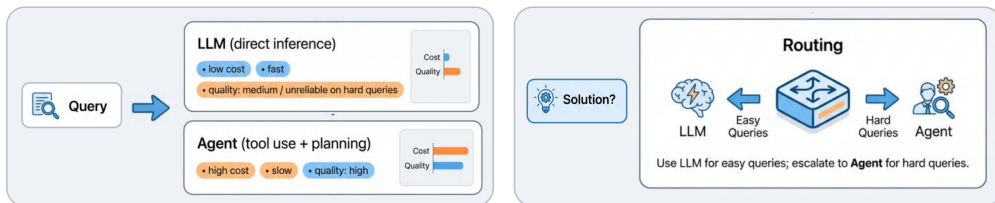
Figure 1: Motivation and overview of routing. Direct LLM inference is fast and low-cost but can be unreliable on harder queries, while full agent execution is slower and more expensive. A router dispatches each query to the appropriate system, using the LLM for easy cases and escalating to the agent when needed to achieve a better accuracy–latency trade-off.
