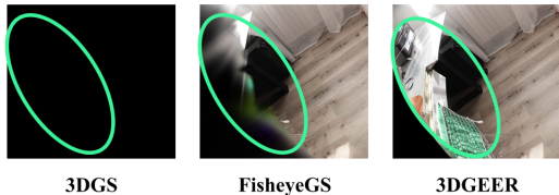
Figure K.1: Out-of-Distribution (OOD) Region in Fig. 6. 3DGS collapses to black due to the numerical issue of \tan 90^\circ \rightarrow \infty , while our method robustly renders views up to 180^\circ , successfully reconstructs the green chair, where splat-based methods (e.g., FisheyeGS) fail. Similarly, in Fig. 6 (zoom-in), our method also preserves structures like the corridor and fridge, table and door, or window and cabinet.
