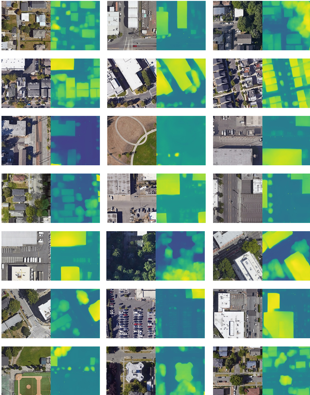
Figure 9: Visual results of our model generated DSM (metric depth) from the monocular satellite image, which is rendered from the satellite view, with no metric depth data for training.
