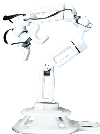
Figure 11: The exoskeleton designed at half scale (1:2) with the same kinematic structure as the Franka arm.
