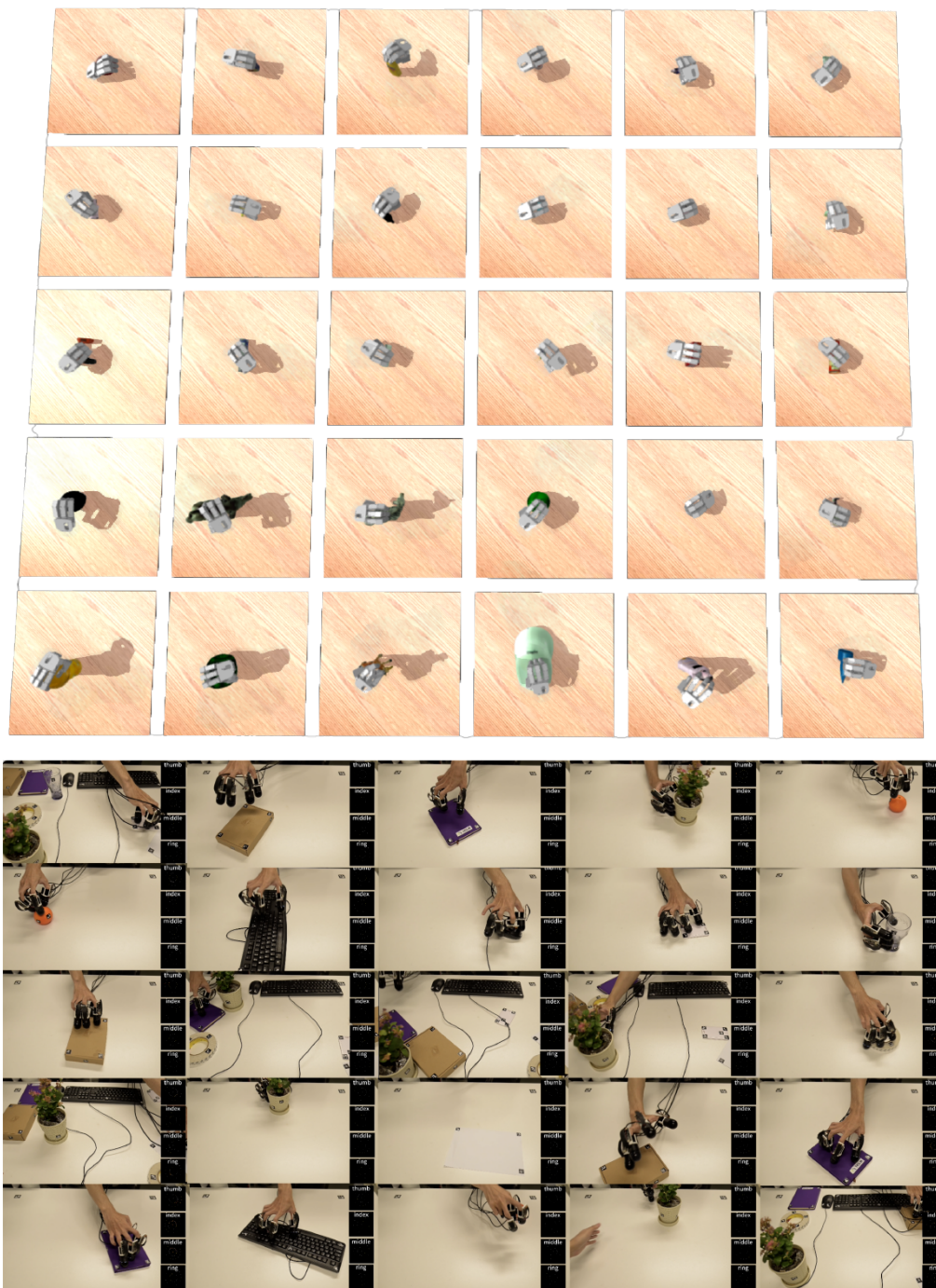
Figure 14: Illustration of the two datasets collected in this work. Top shows the non-prehensile trajectory dataset, bottom depicts the human-demonstrated tactile-force dataset.
