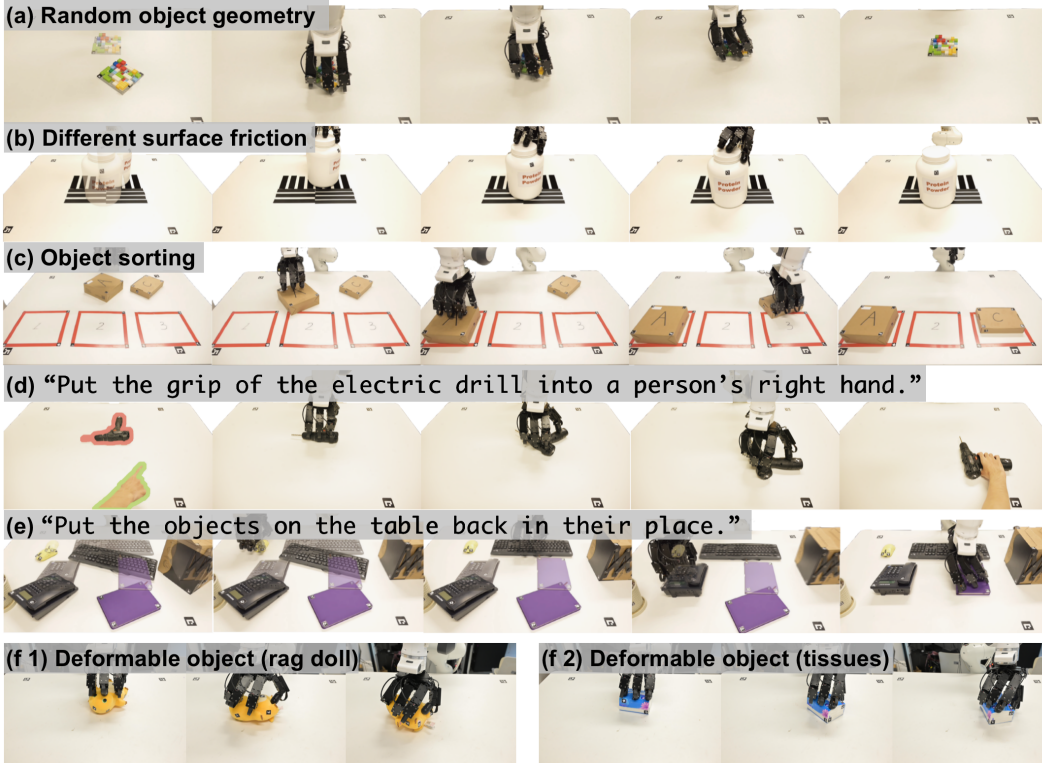
Figure 5: Demonstrations of non-prehensile manipulation. Our learned policy robustly adapts to (a) objects with challenging geometries and (b) varying surface friction. In addition, the learned skill supports reasoning tasks such as (c) object sorting, and language-guided repositioning tasks, including (d) non-prehensile handover and (e) tidying up objects on a desktop, (f) deformable objects (rag dolls and a packet of tissues).
