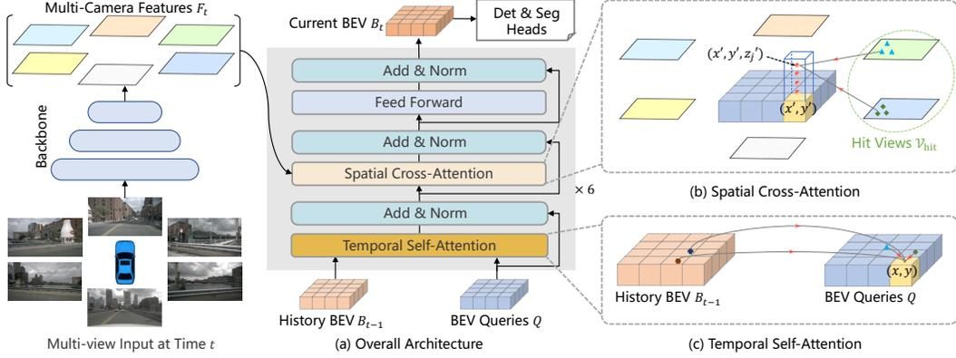
Figure 2: **Overall architecture of BEVFormer.** (a) The encoder layer of BEVFormer contains grid-shaped BEV queries, temporal self-attention, and spatial cross-attention. (b) In spatial cross-attention, each BEV query only interacts with image features in the regions of interest. (c) In temporal self-attention, each BEV query interacts with two features: the BEV queries at the current timestamp and the BEV features at the previous timestamp.
