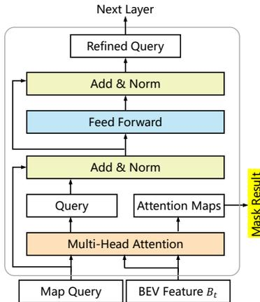
Figure 5: Segmentation head (mask decoder) of BEVFomer.
