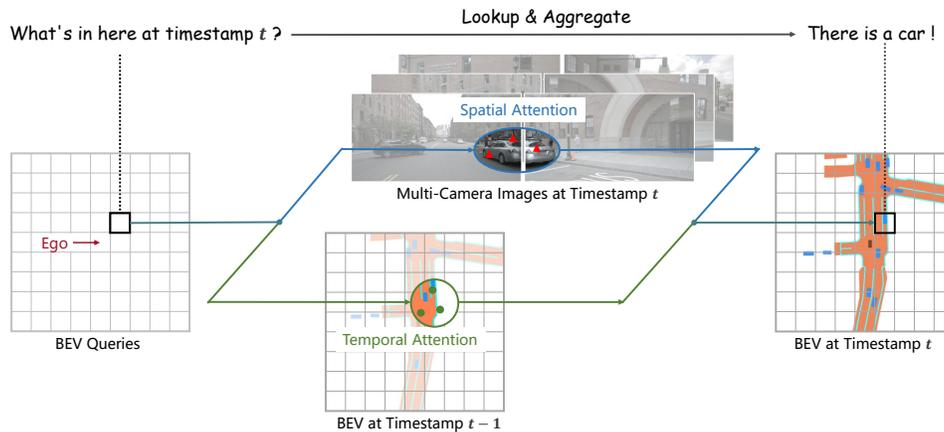
Figure 1: We propose **BEVFormer**, a paradigm for autonomous driving that applies both Transformer and Temporal structure to generate bird’s-eye-view (BEV) features from multi-camera inputs. BEVFormer leverages queries to lookup spatial/temporal space and aggregate spatiotemporal information correspondingly, hence benefiting stronger representations for perception tasks.
