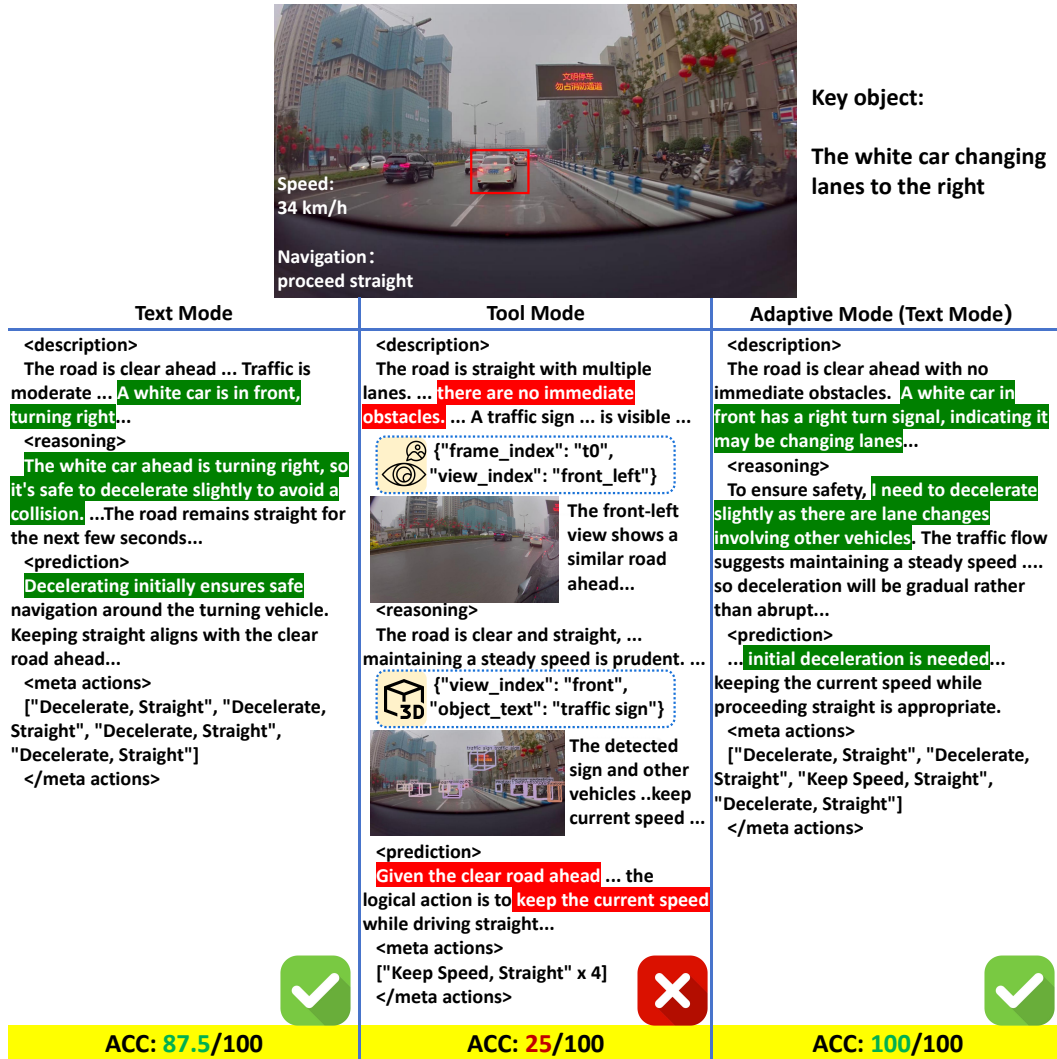
Figure 15: Comparison of reasoning modes in a clear, high-dynamic scenario. The key object is a white car cutting into the ego-lane (top). Center ( \mathcal{M}_{tool} ): When forced to use tools in a clear scenario, the model becomes distracted. It invokes 3D Object Detection for a non-critical traffic sign, introducing irrelevant information that diverts attention from the immediate braking event, leading to a dangerous “Keep Speed” prediction. Right ( \mathcal{M}_{adaptive} ): The model correctly recognizes that the initial visual context is sufficient. It selects Text Mode, avoiding the noise and cognitive load of unnecessary tool calls. By focusing on the clear visual evidence of the cut-in, it correctly predicts the necessary deceleration. This highlights the importance of Hybrid Thinking in preventing “tool abuse” and information overload.
