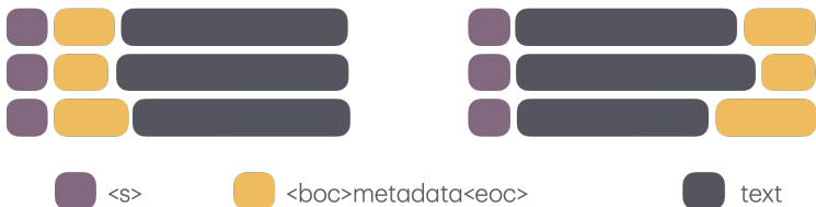
Figure 1: Diagram of our tokenization. Each document begins with a default beginning-of-sequence (<s>) token. For each sequence, metadata is wrapped between beginning-of-context (<boc>) and end-of-context (<eoc>). Depending on the metadata position, the metadata is prepended (illustrated on the left) or appended (illustrated on the right) to the document. If a long document split into multiple sequences, metadata is attached to each one. A 10% dropout of metadata is always performed.
