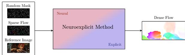
Figure 1: We present a *neuroexplicit* architecture for inpainting of optical flow fields. An *explicit* inpainting model based on partial differential equations (PDEs) is enhanced with *neural* parameter selection. The resulting model inherits both the exceptional out-of-domain generalization from the explicit side and the reconstruction quality from the neural side.
