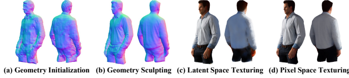
Figure 8: Ablation on Geometry and Texture Reconstruction. (a) shows the geometry initialization, (b) recovers finer details through geometry sculpting, (c) applies latent-space texturing, and (d) achieves the final reconstruction with pixel-space optimization.
