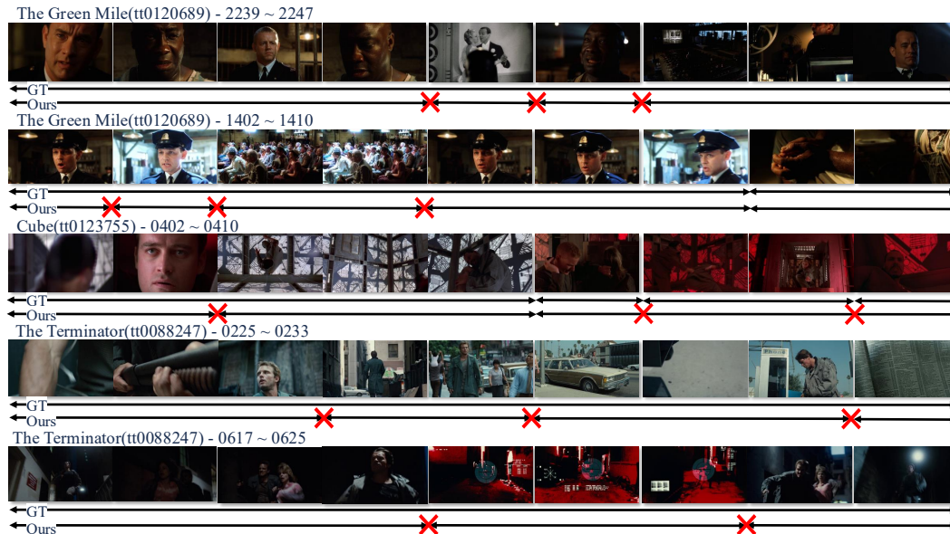
Figure 3: Common failure patterns in scene segmentation. Ground truth (GT) boundaries are shown with black arrows; our predictions with red X marks indicating errors.
