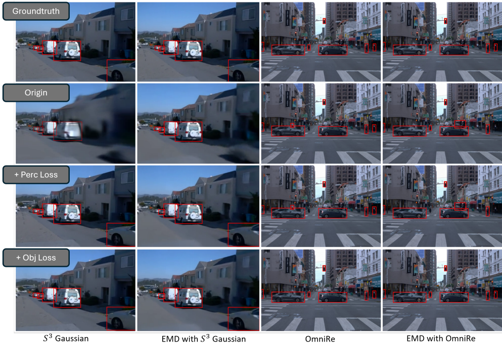
Figure 1: We enhance perception stability in 3D reconstruction by introducing perception-based loss and object zone quality loss, ensuring that the reconstructed images produce perception results consistent with the ground truth for reliable autonomous driving applications. The red box is the bounding box detected by the perception model.
