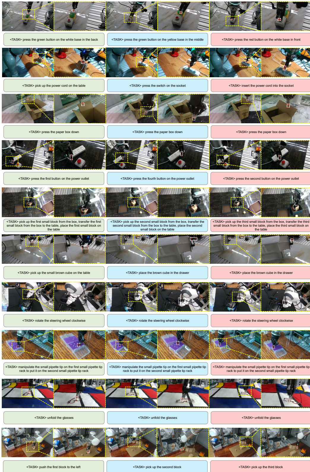
Figure 20: Visualization of contact points (red dots) and contact boxes (white) in multi-task episodes. Each subtask is annotated below, with two images per subtask: a global scene (left) and a zoomed-in interaction view (right).
