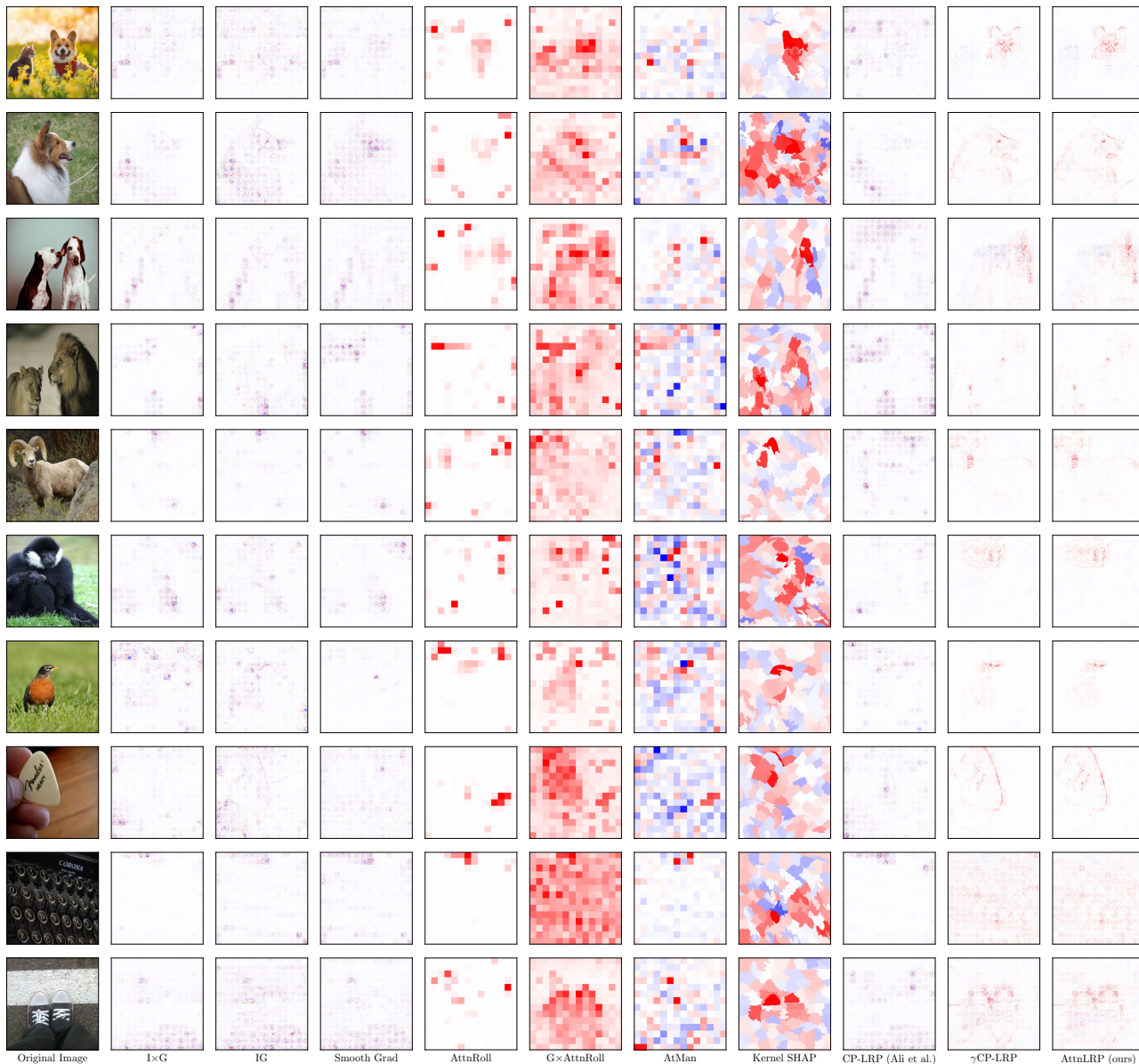
Figure B.6. Explanation heatmaps of the methods used for the perturbation experiments on the vision transformer ViT-B-16. A checkerboard effect is visible for almost every method, especially in AttnRoll (Abnar and Zuidema, 2020), G \times AttnRoll (Chefer et al., 2021a), and AtMan (Deb et al., 2023). We improve upon CP-LRP (Ali et al., 2022) by applying the \gamma -rule as described in B.5. While qualitatively \gamma CP-LRP (with \gamma extension for ViT) and AttnLRP give similar explanations, quantitative results in Table 1 and Table B.6 show a consistent improvement of AttnLRP over \gamma CP-LRP in terms of faithfulness. Moreover, attributing query and key linear layers within the attention layer is possible with AttnLRP only, while it is not possible with CP-LRP. We leave these further explorations for future work.
