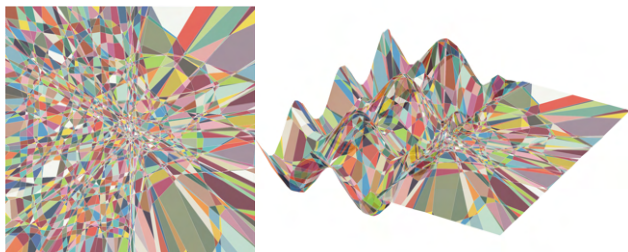
Figure 3. Curvature and complexity. Visual depiction of Equation (2) with a toy affine spline S : \mathbb{R}^2 \rightarrow \mathbb{R} , obtained by training an MLP to regress the piecewise function f(x_1, x_2) = \{\sin(x_1) + \cos(x_2)\} \mathbb{1}_{x_1 < 0} . Regions in the input space partition \Omega (left) and the graph of the affine spline function (right) are randomly colored. The spline partition has significantly higher density of non-linearities for x_1 < 0 , i.e., the local complexity is higher where the learned function has more curvature.
