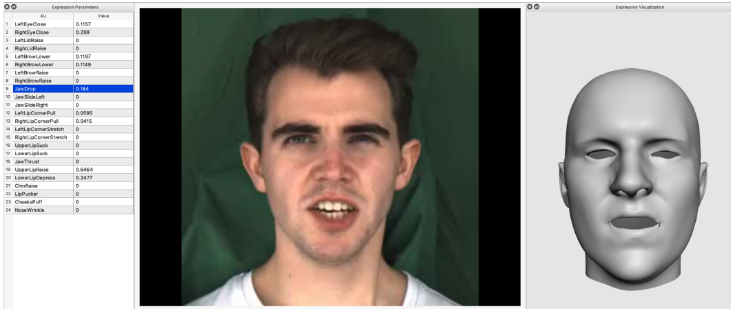
Figure 9: Frame level AU verification interface. Each frame displays the annotated AU values, the original face image, and its mesh based projection, enabling cross-modal consistency checking.
