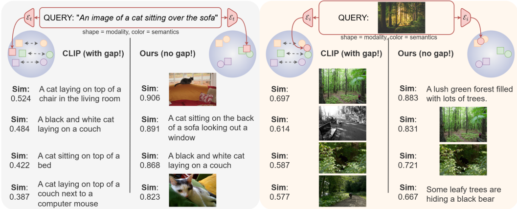
Figure 4: Most similar vectors from the MSCOCO vector databases with both modalities embedded. CLIP learned space has a gap of 0.47 and, for a text query, all the closest embeddings come from the text modality, meaning that embeddings are clustered according to the modality and not according to the overall multimodal semantics. On the contrary, the proposed method has nearly a zero gap, and most similar samples come from both the image and text modalities, proving that we can effectively build a multimodal latent space that is semantically coherent among the modalities. The same behavior holds for an image query.
