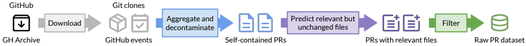
Figure 6: Overview of SWE-RL’s raw pull request data curation process. The collected git clones and GitHub events are transformed into self-contained PR instances via decontamination, aggregation, relevant files prediction, and filtering.
