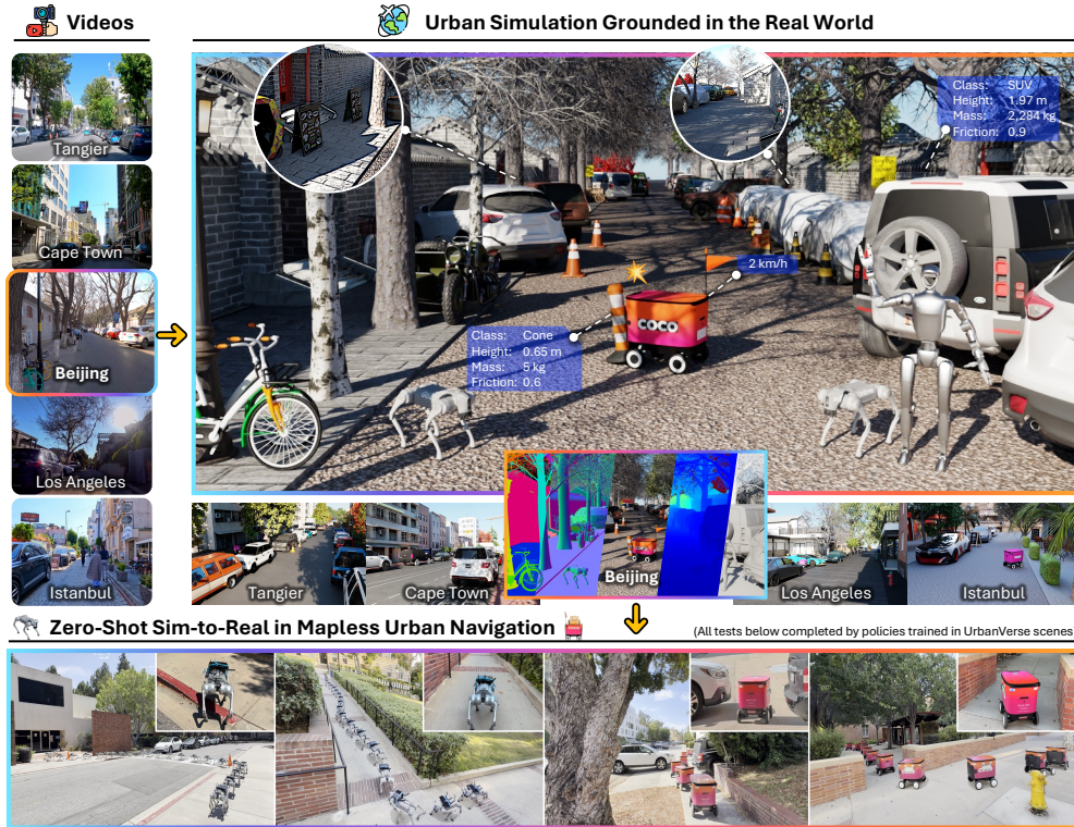
Figure 1: UrbanVerse system converts real-world urban scenes from city-tour videos into physics-aware, interactive simulation environments, enabling scalable robot learning in urban spaces with real-world generalization.
