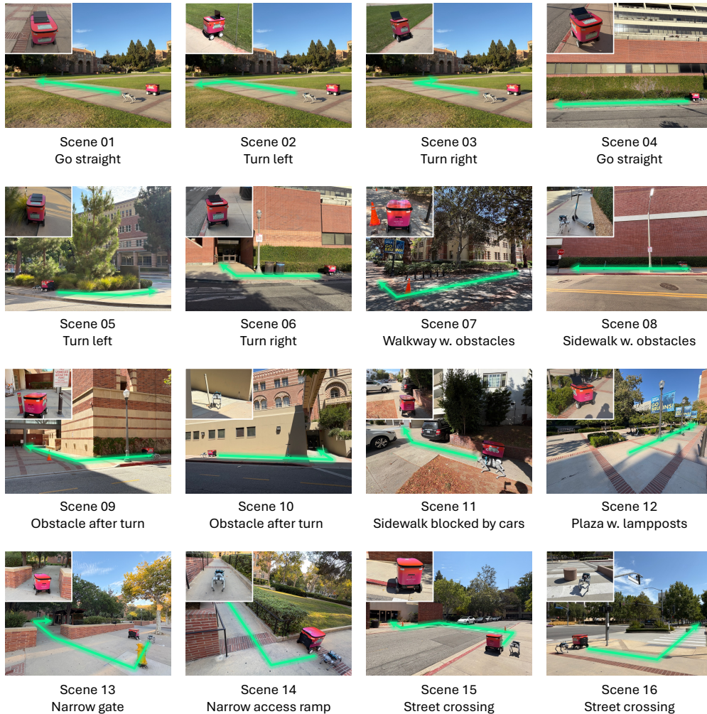
Figure 35: Real-world testing scenarios. We evaluate zero-shot sim-to-real policy transfer across 16 diverse urban scenes and two embodiments (Coco wheeled delivery robot and Unitree Go2 quadruped), spanning challenges such as straight paths (Scenes 01, 04) and turns (Scenes 02, 03, 05, 06) on open ground or sidewalks, walkway and sidewalk obstacles (Scenes 07, 08), obstacles appearing after turns (Scenes 09, 10), sidewalk blockage by cars (Scene 11), structural elements including lampposts and narrow access points (Scenes 12–14), and street crossings (Scenes 15, 16). Key challenges for each scene are highlighted in Red at the upper-right corner.
