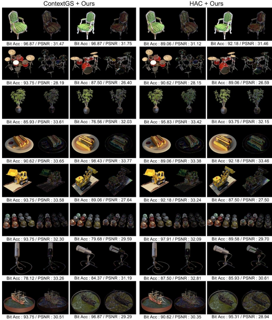
Figure 20: Rendering quality of various rendering outputs generated by our method on the Blender dataset. We show the differences ( \times 5 ). The closer it is to white, the greater the discrepancy between the ground truth and the rendered image. The results were obtained using 64-bit messages after compression.
