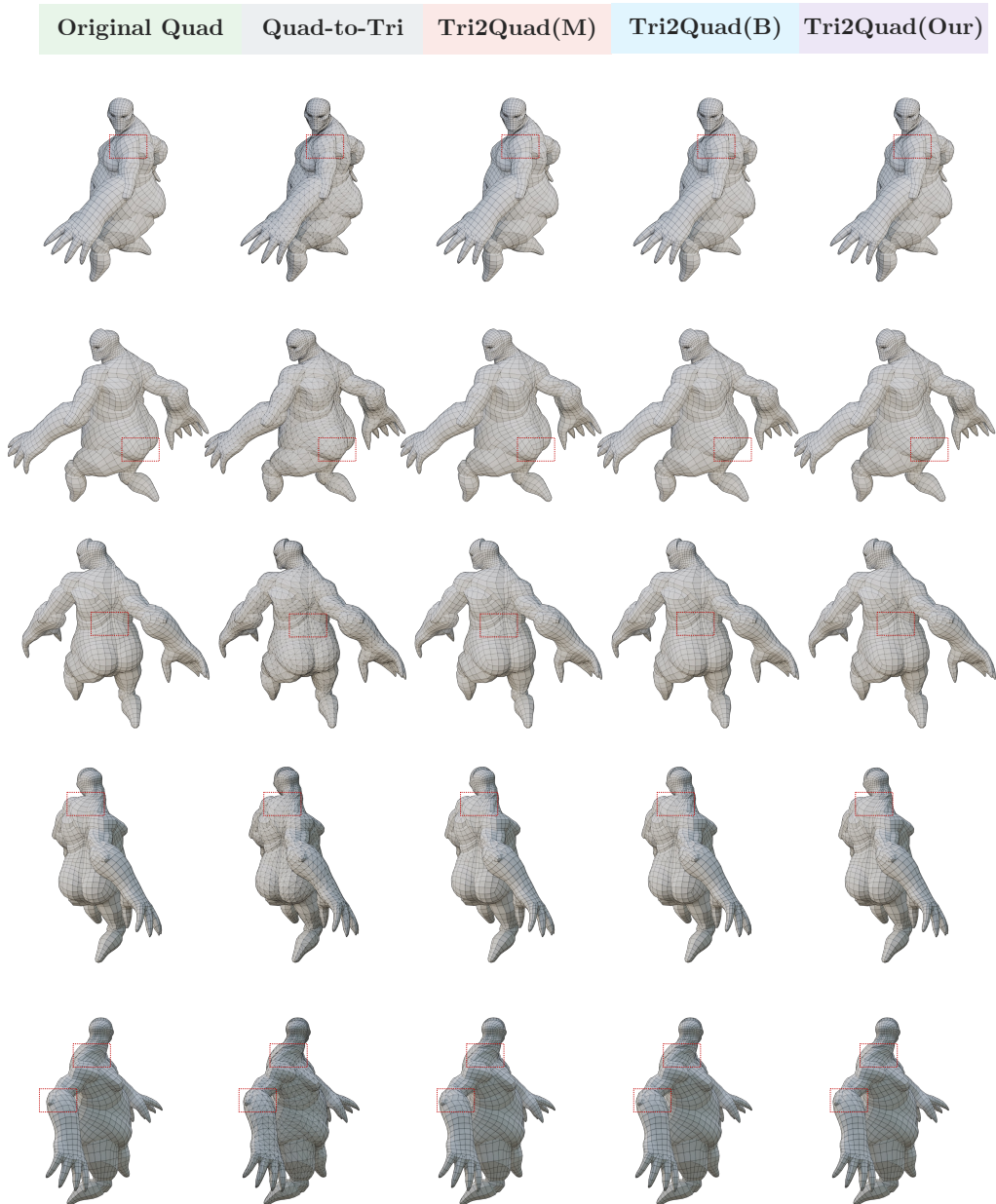
Figure 14: The Irreversibility of Triangulation and Limitations of Conversion Algorithms. (a) A high-quality artist-created quad mesh with clean edge flow. (b) The same mesh after triangulation—the ground truth topological information is now ambiguous. (c-e) The results of applying different tri-to-quad conversion algorithms to (b). While our ILP-based operator (e) produces a better result than the default methods in MeshLab (c) and Blender (d), none can perfectly recover the original topology, resulting in broken edge loops and artifacts. This demonstrates the fundamental limitations of post-hoc conversion.
