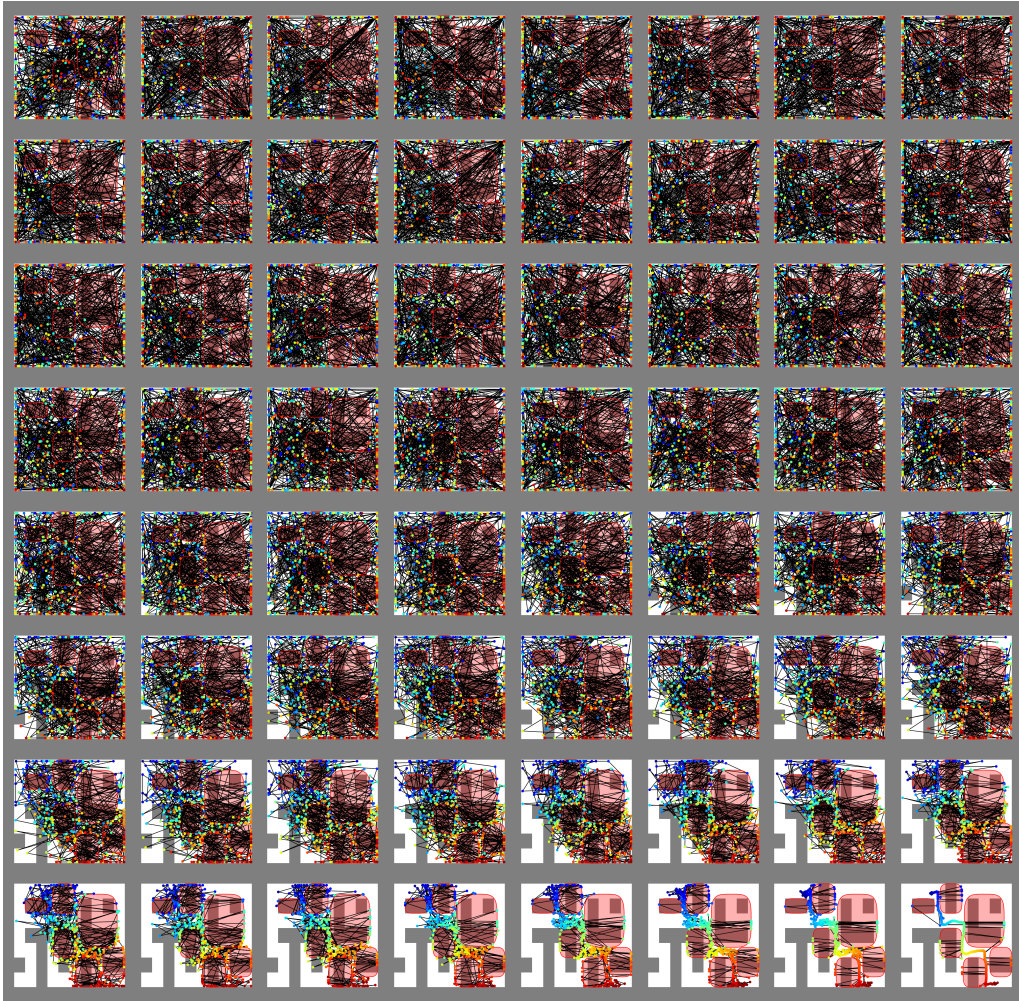
Figure 17: Path Generation Process of SafeDiffuser (Xiao et al., 2025) in Maze2D environment with six constraints. From the top-left to the bottom-right, we visualize \tau_t on a uniform time discretization of [T, 0] , excluding the midpoint t = 0.5T .
