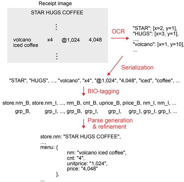
Figure 1: The scheme of post-OCR parsing task.
