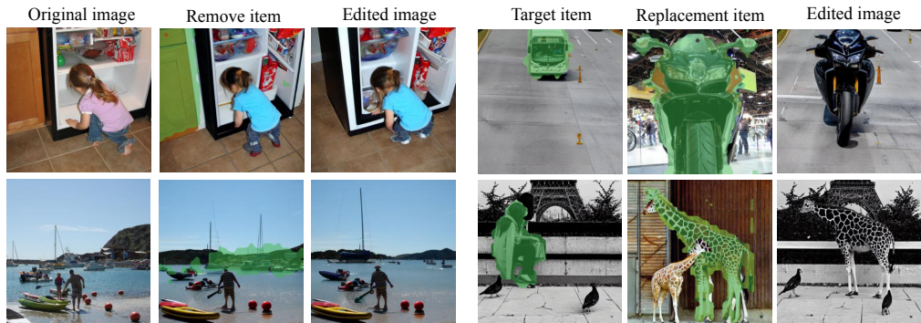
Figure 3: Illustration of compositional editing. CODA can compose novel scenes from real-world images by removing (left) or swapping (right) the slots, shown as masked regions in the images.
