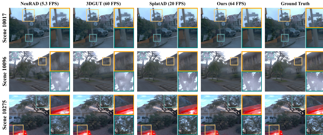
Figure 5: Static NVS. Projecting LiDAR as a sparse depth map causes inaccuracies that degrade 3DGUT’s rendering of the pole ( above ), which we avoid by rendering LiDAR directly. Our bilateral grids also prevent floaters ( middle ), allowing us to render slightly faster. SplatAD’s CNN does not properly recover the sign lettering ( above ) or rear car seat ( below ), while our simpler pipeline does.
