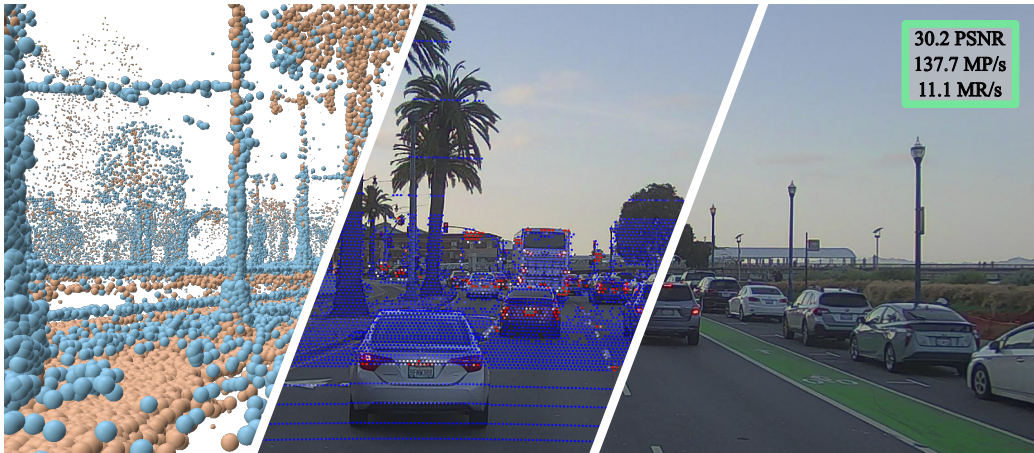
Figure 1: SimULi . We design a factorized 3D Gaussian representation that encodes camera and LiDAR information into separate sets of 3D Gaussians joined via nearest-neighbor anchoring loss ( left ). To efficiently render LiDAR scans ( middle ), we extend 3DGUT (Wu et al. 2025b) with an automated tiling strategy and ray-based culling. When compared to existing methods, we render 1.5-20 \times faster and match or exceed LiDAR and camera quality ( right ) across a wide range of metrics.
