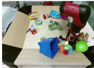
Figure 1: The video prediction model is trained on 17,000 video sequences collected autonomously by a Sawyer robot interacting with 140 different every-day objects.
