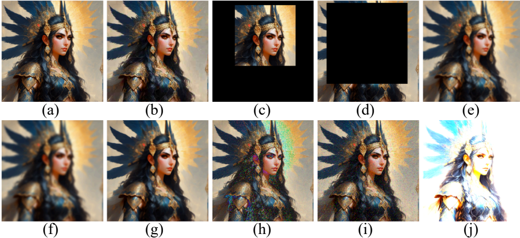
Figure 6: Visualization of the distortion set used in our experiments. (a) Clean image or identity transformation. (b) JPEG, QF = 25 . (c) 60% area Random Crop (R.Crop). (d) 80% area Random Drop (R.Drop). (e) 25% Resize and restore (Resize). (f) Gaussian Blur, r = 4 (G.Blur). (g) Median Blur, k = 7 (M.Blur). (h) Gaussian Noise, \mu = 0 , \sigma = 0.05 (G.Noise). (i) Salt and Pepper Noise, p = 0.05 (S&P). (j) Brightness, factor = 6 (Bright).
