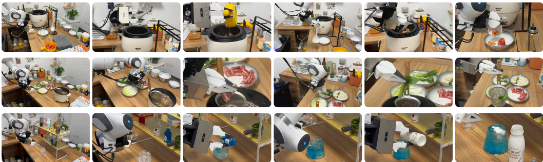
Figure 8: Execution processes of three long-horizon tasks: Tomato-Egg, Hotpot, and Cocktail (exemplified by Mountain Fuji preparation).
