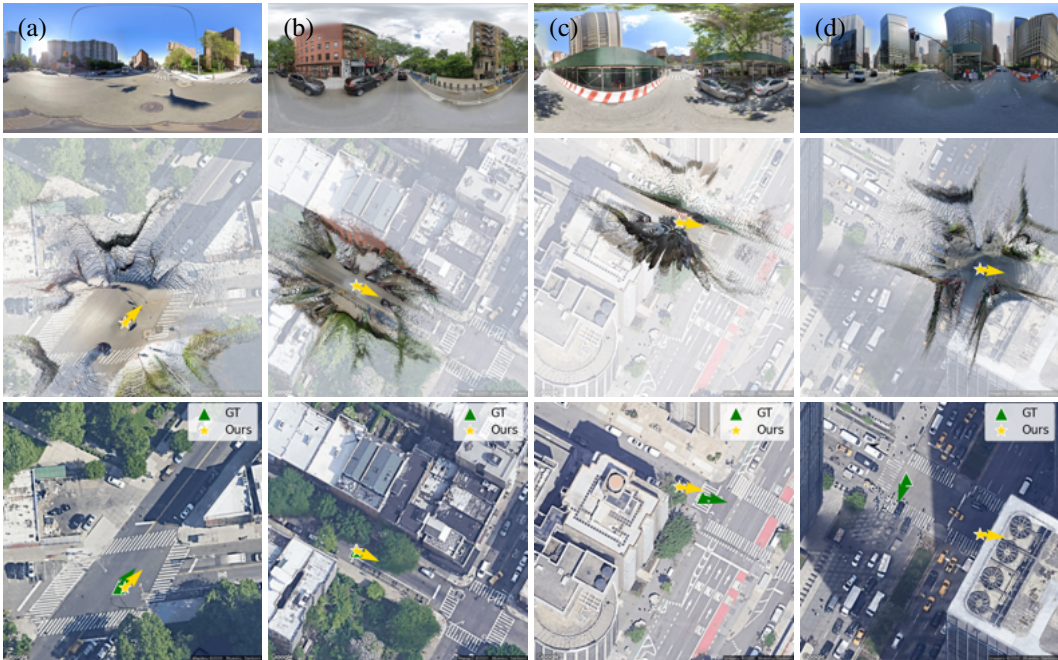
Figure 5: Ground layout overlaid on the aerial image after applying the predicted rotation, translation, and scale transformations. The alignment directly reflects localization quality: the first three examples show successful localization, while the last one illustrates a failure case. Notably, the alignment in example (c) helped us to identify the error in ground truth location.
