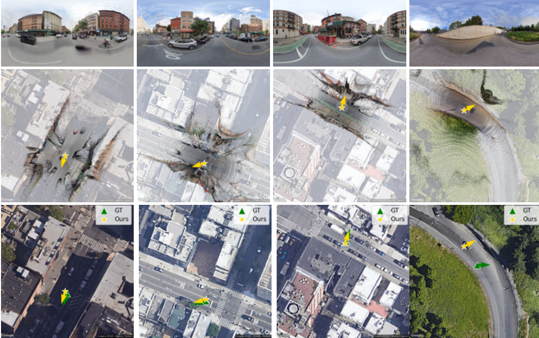
Figure 13: Ground layout overlaid on the aerial image after applying the predicted rotation, translation, and scale transformations. The alignment directly reflects localization quality: the first three examples show successful localization, while the last one illustrates a failure case. Relative depth is obtained from BiFuse++ (Wang et al., 2022).
