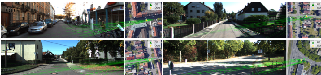
Figure 9: Success cases for localization on the KITTI same-area test set under \pm 10^\circ orientation noise. We visualize the top 50 correspondences, ranked by matching score
