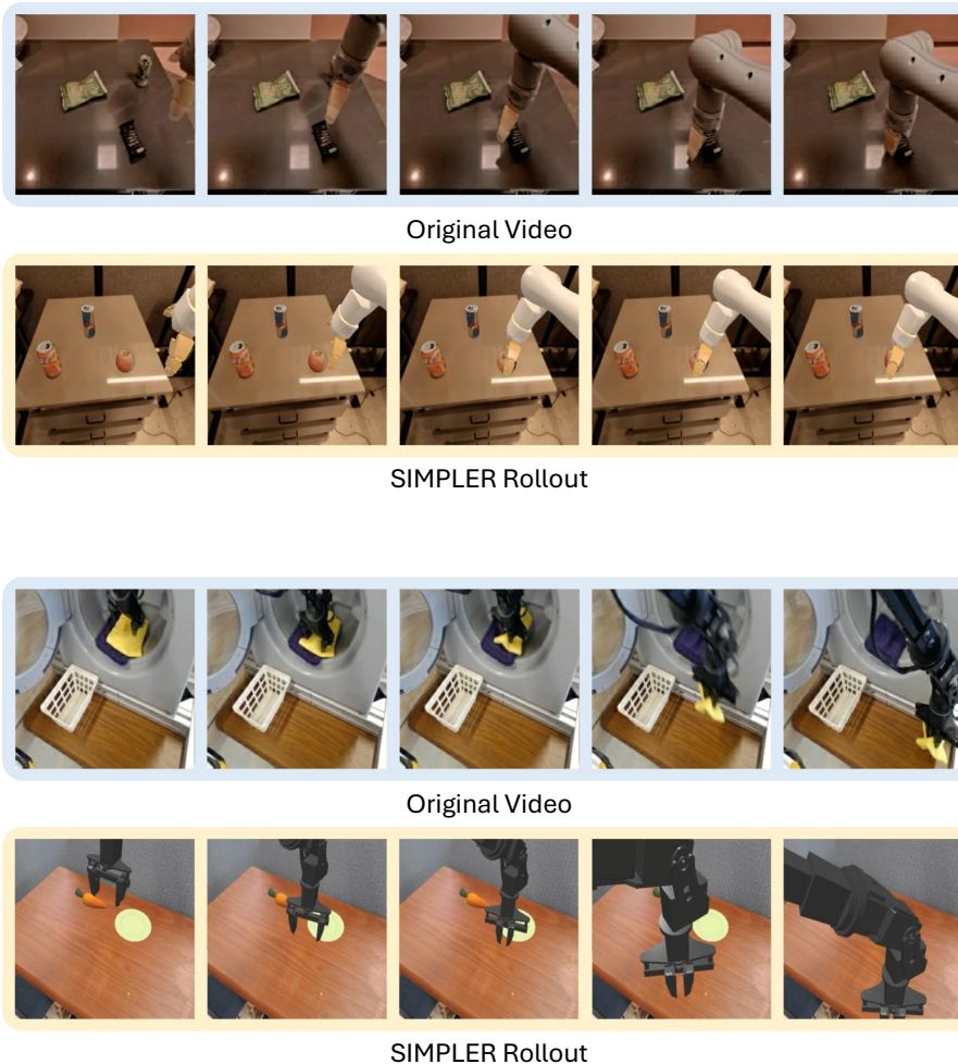
Figure 7: Transfer robot video demonstrations into robot actions through LAM and proprio FDM in SIMPLER simulator. Upper: the SIMPLER rollout closely reproduce the motion of moving downwards, Bottom: the SIMPLER rollout closely reproduce the motion of moving right.
