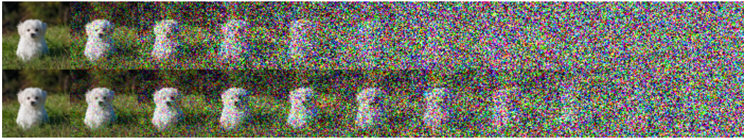
Figure 2: Latent samples from linear (top) and cosine (bottom) schedules respectively at linearly spaced values of t from 0 to T . The latents in the last quarter of the linear schedule are almost purely noise, whereas the cosine schedule adds noise more slowly
