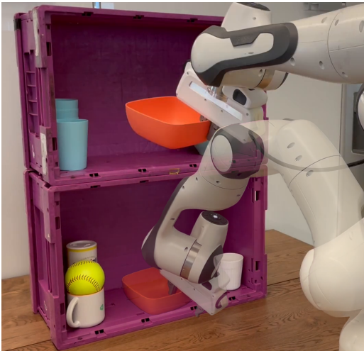
Figure 1: CabiNet is able to perform complex rearrangement tasks in novel, cluttered scenes from just partial point cloud observations without object or environment models.
