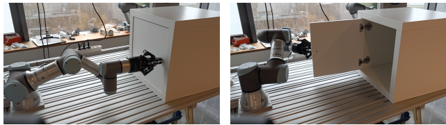
Fig. 1: We create a system to open articulated objects using only the proprioceptive information during contact and find that it can open various articulated objects, such as this IKEA cabinet. This confirms that proprioceptive information is valuable for articulated object manipulation.
