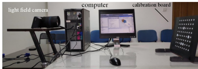
Fig. 5. Light field camera and calibration board.
