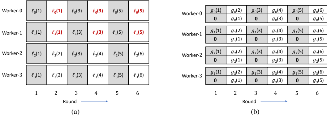
Figure 12: Consider parameters \{n = 4, B = 1, W = 2, \lambda = 4\} ; (a) SR-SGC scheme: reattempted tasks are indicated in red (b) M-SGC scheme.
