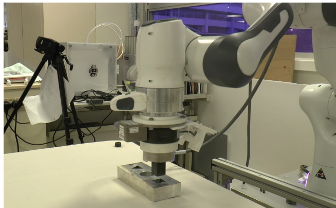
Fig. 1: Robotic assembly setup. A square peg was used in this study.
