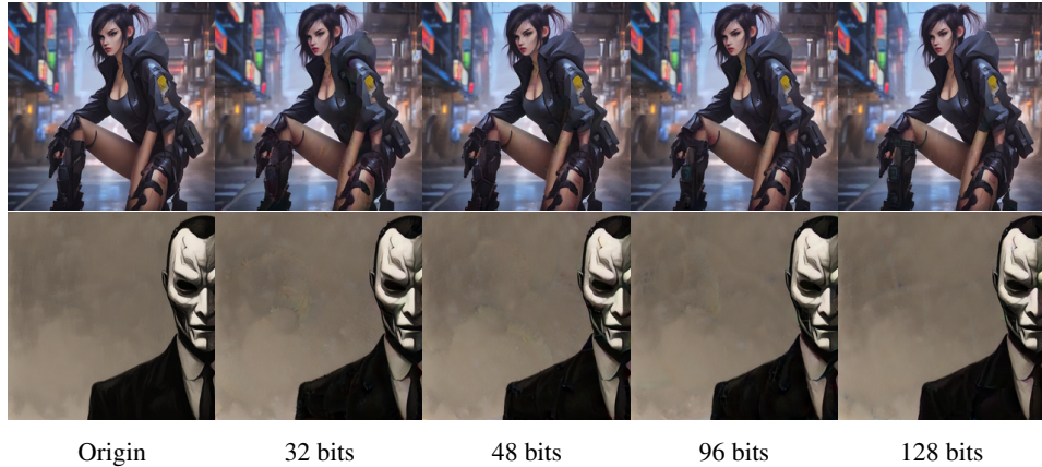
Figure 9: Examples of watermarked images with various encoding bits. FreqMark maintains image quality (approximately 31 dB in terms of PSNR) without degradation as the number of encoding bits increases while the bit accuracy against regeneration and Gaussian noise attacks may be reduced. Encoding 48 bits is the default setting.
