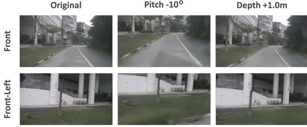
Figure 3. Camera images under different viewpoint perturbation conditions. Each column shows the Original, Pitch -10^\circ , and Depth +1.0 m conditions for the front and front-left cameras.
