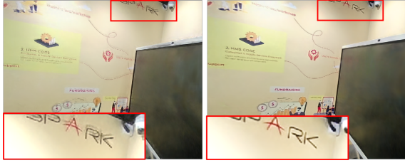
Figure 7. Qualitative examples for novel view synthesis with (right) and without (left) intrinsic refinement. We eliminate blurriness and enhance rendering quality by refining camera intrinsics during optimization.
