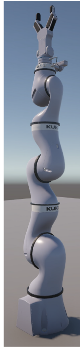
Figure 1: An example of a virtual robotic arm with the 1D pixel layout visualization added. For each joint, a pixel band is added.
