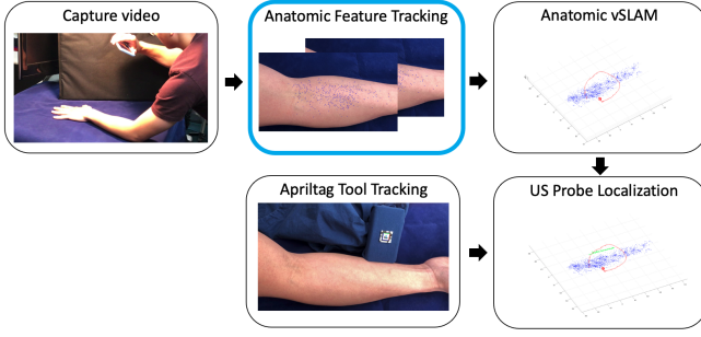
Fig. 1: We incorporate our novel anatomic feature tracking algorithm into an end-to-end 3D tracking and reconstruction system. The blue box indicates our chief contribution to the system. The reconstructed 3D arm features, tracked tool (i.e. AprilTag), and computed smartphone camera trajectory are depicted as blue, red, and green dots, respectively.
