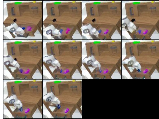
(b) An example of the Lift Blue Block Drawer Task. The gripper arm is entangled with the block.
