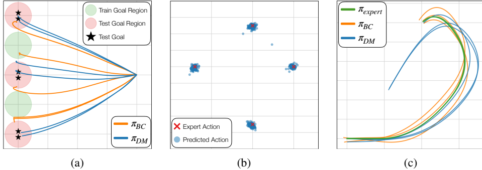
Figure 4: Comparing Modeling Conditional Probability and Joint Probability. (a) Generalization. We collect expert trajectories from a PPO policy learning to navigate to goals sampled from the green regions. Then, we learn a policy \pi_{BC} to optimize \mathcal{L}_{BC} , and another policy \pi_{DM} to optimize \mathcal{L}_{DM} with a diffusion model trained on the expert distribution. We evaluate the two policies by sampling goals from the red regions, which requires the ability to generalize. \pi_{BC} (orange) struggles at generalizing to unseen goals, whereas \pi_{DM} (blue) can generalize ( i.e. , extrapolate) to some extent. (b)-(c) Manifold overfitting. We collect the green spiral trajectories from a script policy, whose actions are visualized as red crosses. We then train and evaluate \pi_{BC} and \pi_{DM} . The trajectories of \pi_{BC} (orange) can closely follow the expert trajectories (green), while the trajectories of \pi_{DM} (blue) deviates from expert’s. This is because the diffusion model struggles at modeling such expert action distribution with a lower intrinsic dimension, which can be observed from incorrectly predicted actions (blue dots) produced by the diffusion model.
