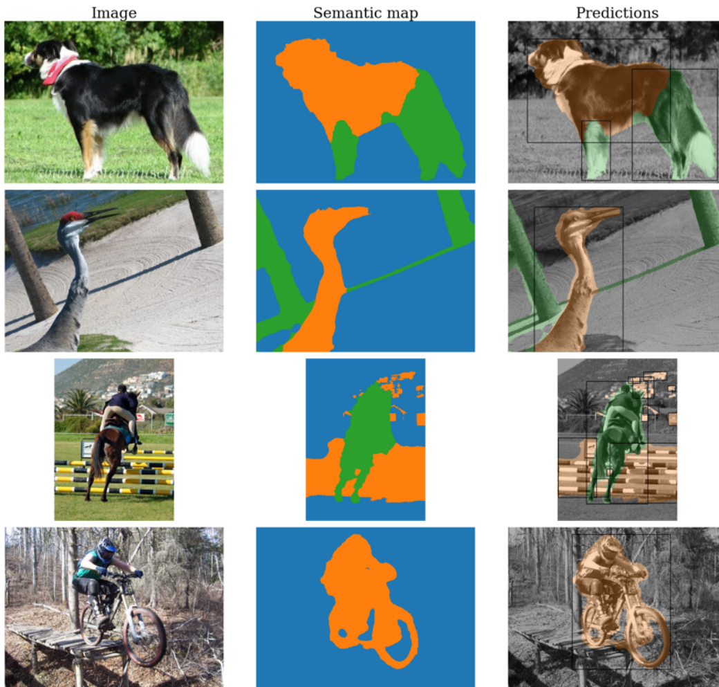
Figure S8: Examples of failure modes in the unsupervised segmentation workflow. First row: over-decomposition of foreground object into legs and body - this can be improved by increasing the merging threshold distance, but can also merge more unrelated classes. Second row: merging of unrelated classes i.e. the shadow of an object and the object. Third and fourth row: over-merging objects close in space i.e. the rider and the horse/bike.
