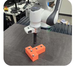
(c) Push-T real-world setup, with a FR3 arm, custom end-effector, and Mocap markers.
