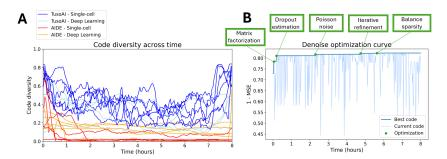
Figure 2: **Behavior of code generated by TusoAI.** (A) Code diversity of TusoAI and AIDE over optimization time, as measured by 1- cosine similarity. Each line corresponds to a dataset. (B) Performance of the current code and the best code over optimization time for a representative task "Denoise". Key optimization changes with their occurrence times are annotated.
